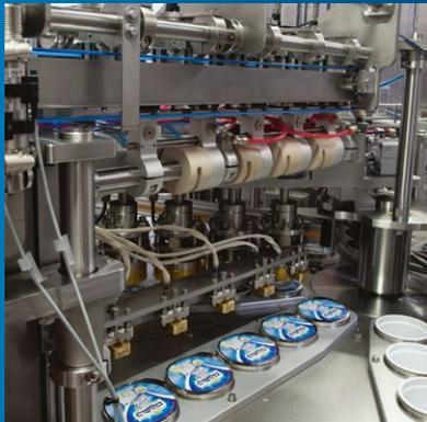
The units are tailor-made to suit your specific needs. Primoreels® deliver a complete lidding solution, with both the dispensing system and the lids used in the system. Primoreels® systems have their own touch screen panels and controls, making them independent units.
