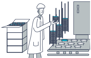
Continuous check and refill of lids magazines
